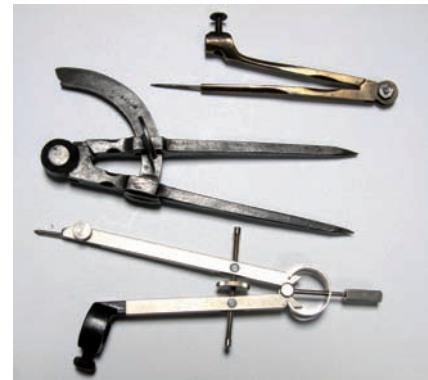
The tools of the geometer from different periods. A schoolchild's serviceable instrument, a mason's tool and a modern draughtsman's tool — all simple compasses.
